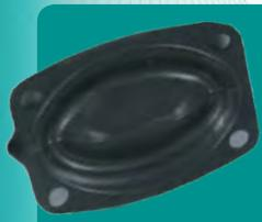
ETHYLENE PROPYLENE (EPDM) -30 degrees to +300 degrees F EPDM is the most popular general purpose material. It possesses excellent chemical resistance to a wide variety of corrosive elements including acids, caustics, and hot water. EPDM is abrasion resistant, good for high temperature service, and is satisfactory for intermittent steam sterilization, but has poor oil resistance.
